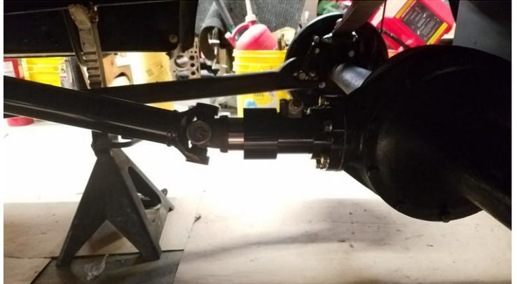
Drive shaft attached to the pinion shaft
