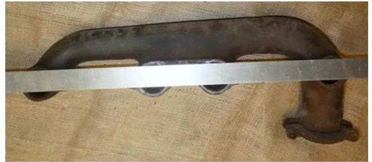
1931 exhaust manifold with the extra reinforcing rib on #4. Notice that there is no sag on #4. All 4 gaps on the top and bottom of the straight edge are the same.
