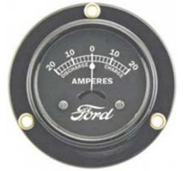
The ammeter in a Model A Ford can be a very useful tool in a variety of situations that will signal to the driver the car's electrical status. Whenever you park a Model A and are about to exit the car, glance at the ammeter, the needle should be pointing to zero. If instead it is pointing slightly to the left it is telling you that somewhere within the car there is some unauthorized current flowing that is going to drain the battery if you leave it that way long enough.
