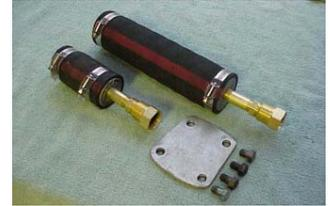
To back flush the radiator, connect the adapters to the two radiator hose bibs. With a garden hose connected to the bottom hose bib adapter run water though the radiator backwards to the normal flow. Be sure to put the radiator cap on. A suggestion, connect the garden hose to your laundry machine hot water spigot and back flush with hot water. A second garden hose may be connected to the top radiator hose bib adapter to carry the exiting water to a suitable drain.
