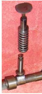
*Jim Morley installed stainless steel valves and valve guides and replaced the double lock lifters with single lock lifters. Proper adjustment eliminated an annoying tapping sound.*
