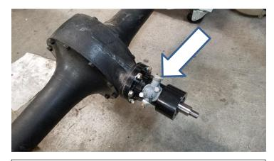
New pinion housing installed on rear end; the little gray item on top is the speedometer drive
