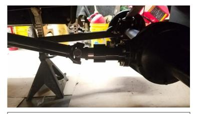
Drive shaft attached to the pinion shaft
