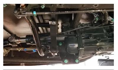
Transmission mounted under car; the brake cross shaft is mounted 1" forward of the E brake shaft
