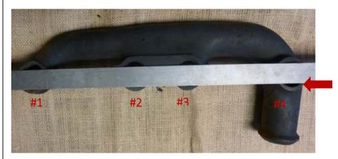
Problem: #4 port has sagged in relation to the other three ports. Notice the 1/4" gap on #4 port indicated by the arrow when the straight edge is aligned with the lower edge of the first three exhaust ports. This sag on #4 is caused by the combination of heat and the weight of the exhaust pipe. This manifold will never bolt up to a block when using the correct exhaust manifold gland rings. I also checked two other original manifolds: same problem.
