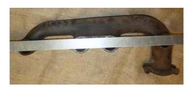
1931 exhaust manifold with the extra reinforcing rib on #4. Notice that there is no sag on #4. All 4 gaps on the top and bottom of the straight edge are the same.
