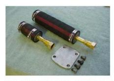
Shown above are the two adapters and the water pump blanking plate. The long hose is the upper (larger diameter) hose. The short hose is the lower (smaller diameter) hose.
